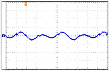
Figure 10: Output Voltage Ripple, Vout, at nominal input voltage and rated load current. Load capacitance:  $1\mu F$  ceramic capacitor and  $100\mu F$  electrolytic capacitor. Bandwidth: 20 MHz (See Figure 13). Ch 1: Vout (100mV/div), Time (2uS/div).
