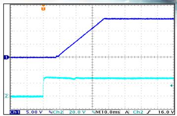
Figure 8: Turn-on transient at full resistive load and zero output capacitance initiated by Vin. ON/OFF Pin previously low. Ch 1: Vout (5V/div), Ch 2: Vin (20V/div), Time (10mS/div).
