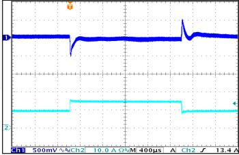
Figure 11: Output Voltage Response to Step-Change in Load Current (50%-75%-50% of Iout(max); di/dt = 5  $A/\mu s$ ). Load cap:  $1 \mu F$  ceramic and  $100 \mu F$  electrolytic capacitors. Ch 1: Vout (500mV/div), Ch 2: Iout (10A/div), Time
