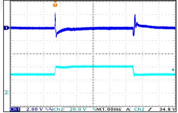
Figure 12: Output Voltage Response to Step-Change in Input Voltage (250V/mS). Load cap: 100 µF electrolytic output capacitance. Ch 1: Vout (2V/div), Ch 2: Vin (20V/div), Time (1mS/div).
