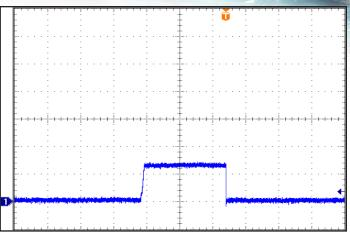
Figure 14: Output Short Load Current as a function of time when the converter attempts to turn on into a 10 m $\Omega$  short circuit. Ch 1: Load current (20A/div), Time (20mS/div).
