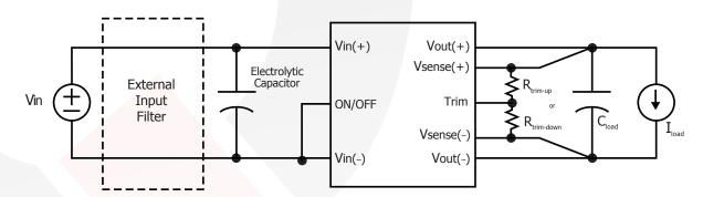
Figure C: Typical Application Circuit (negative logic unit, permanently enabled).
