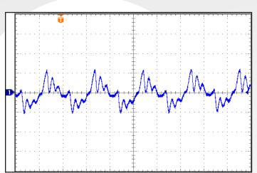
Figure 9: Input Terminal Current Rpple, i<sub>C</sub> at full rated output current and nominal input voltage with 220uF electrolytic capacitor. Bandwidth: 20MHz (See Figure 13). Ch 1: Input current (1A/div), Time (2uS/div).
